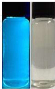
Photos of GO quantum dots solution at 365 nm UV lamp (left) and under natural light (right)
