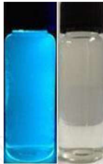
Photos of GO quantum dots solution at 365 nm UV lamp (left) and under natural light (right)
