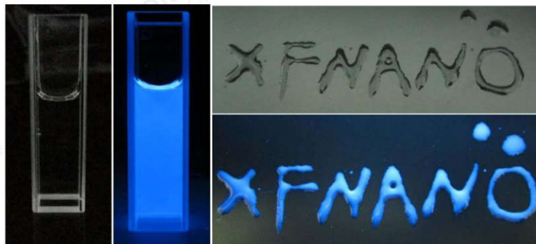
Photos of Aminated Graphene quantum dots N-150 under natural light and at 365 nm UV lamp
